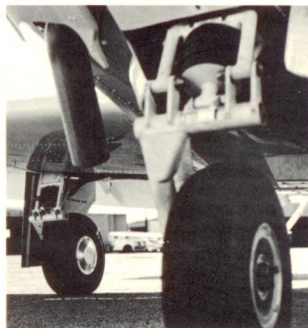
Rugged Mooney gear has no fancy hydraulics or oleos to run up shop bills. Positive-action energy-absorbing electric gear retracts in three seconds, extends in two.
